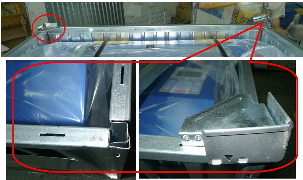
Step 4: Fix the four side boards by four corner brackets.
